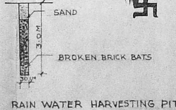
RAIN WATER HARVESTING PIT
